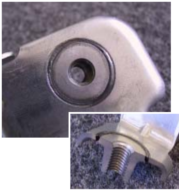
Zn coated, 1,8 mm thickness 30mm/s, 3,5 kW, Helium
